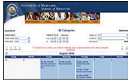
(Ex. 2) - Webpage at 100% wide. The browser is maximized to a viewing area of approximately 1000 pixels. Components within the Calendar automatically expand to fill the width. As the browser decreases in size the components will adjust accordingly.
